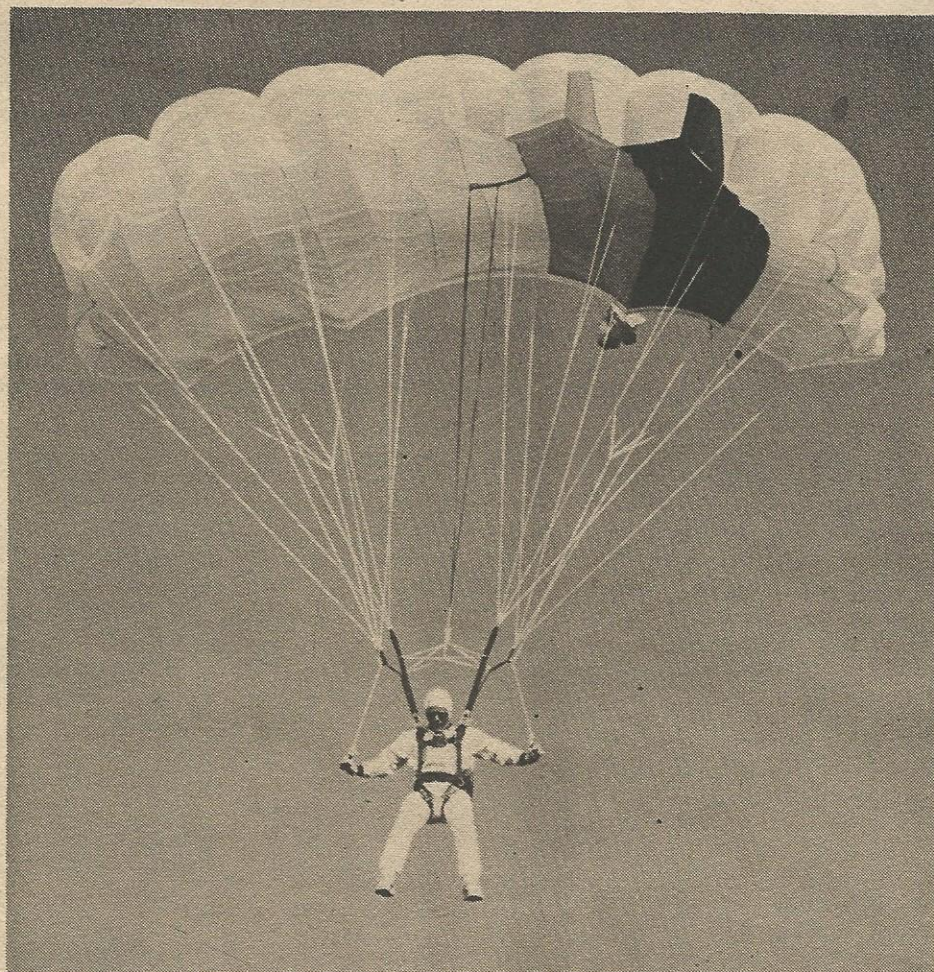
Bill Wenger of Pioneer Parachute Company demonstrates Pioneer's new 265-sq. ft. Titan canopy. The canopy shown here is equipped with a high-speed reefing system designed for style jumpers and military applications. The Titan is comparable in size to the Para-Flite XL Cloud and the GQ Security Unit 3. Weight with risers is reported to be 10.4 lbs. Slider deployment is standard. Pioneer photo.
